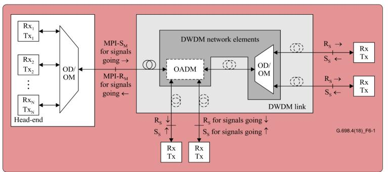
The tail-end equipment (TEE) transmitters have the capability to adapt their DWDM channel frequency to the optical demultiplexer/optical multiplexer (OD/OM) or OADM port they are connected to using feedback from the head-end equipment (HEE) via the head-to-tail message channel (HTMC).
