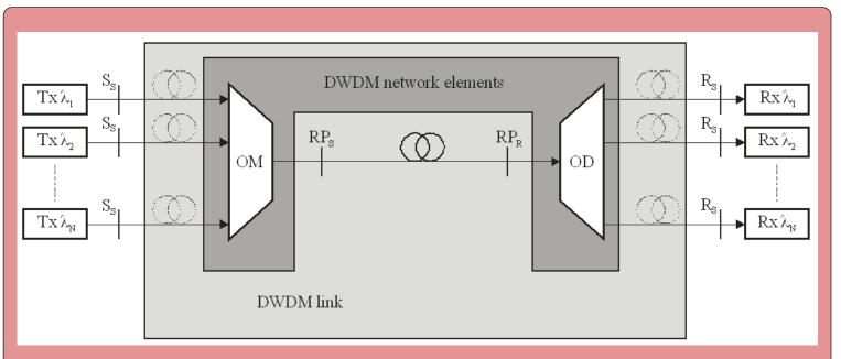
Physical point-to-point WDM applications in the O-band on single-mode optical fibres through the use of the "black link" approach
