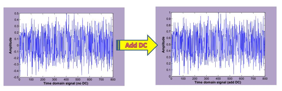
Light intensity must be *unipolar* and *non-negative*. Directed circuit (DC) should be added.
