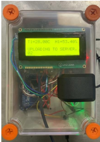
Sensor (temperature, RH, ethylene) based system
