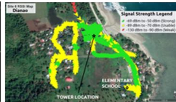
Sample RSSI Mapping using Network Monitor Lite.
