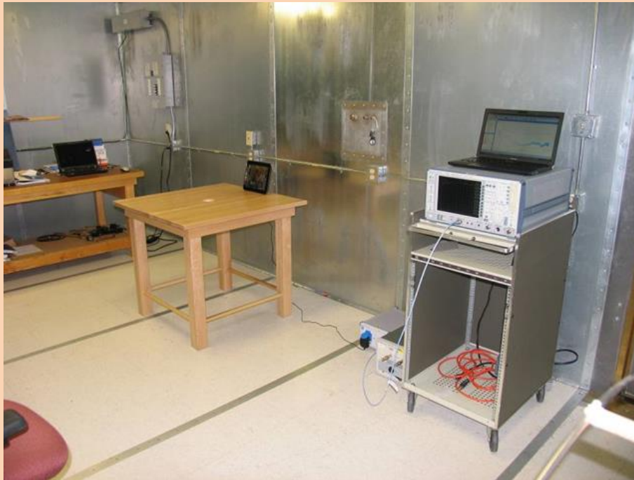
Figure 14: Shielded room inside view
