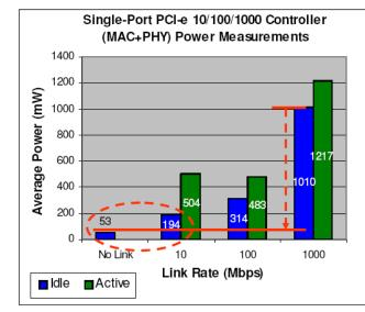
Source: Intel labs. Intel® 82573L Gigabit Ethernet Controller, 0.13µm, "Idle" = no traffic, "Active" = line-rate, bi-directional
