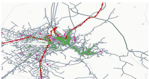
Figure A1.5. Fibre network with power grid overlay can identify routes for expansion
