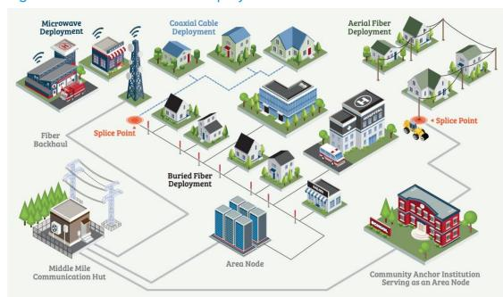
Figure 23. Common network deployments
