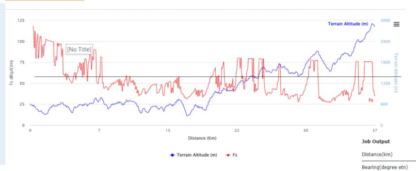
Study FS variation on the path from TX to a RX point in the contours farthest from the TX in the P2A coverage analyses
