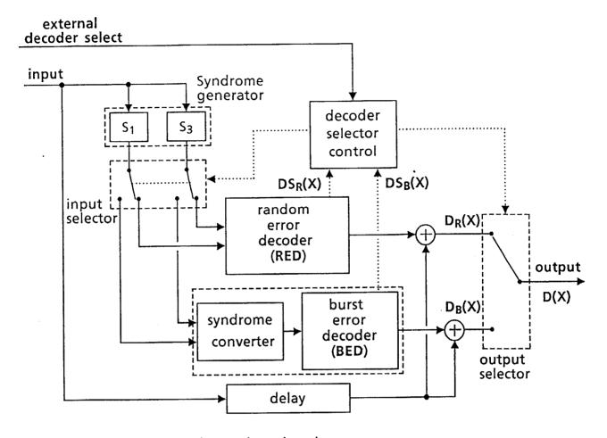
D<sub>R</sub>(X) decoded signal by random decoder
