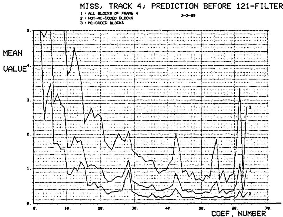
Figure 10: Average Value of the DCT Coefficients Subblocks fourth track of the Miss America sequence before the prediction filter
