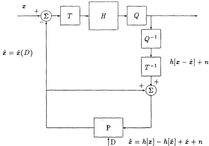
Figure 4: Filtering without feedback filtering
