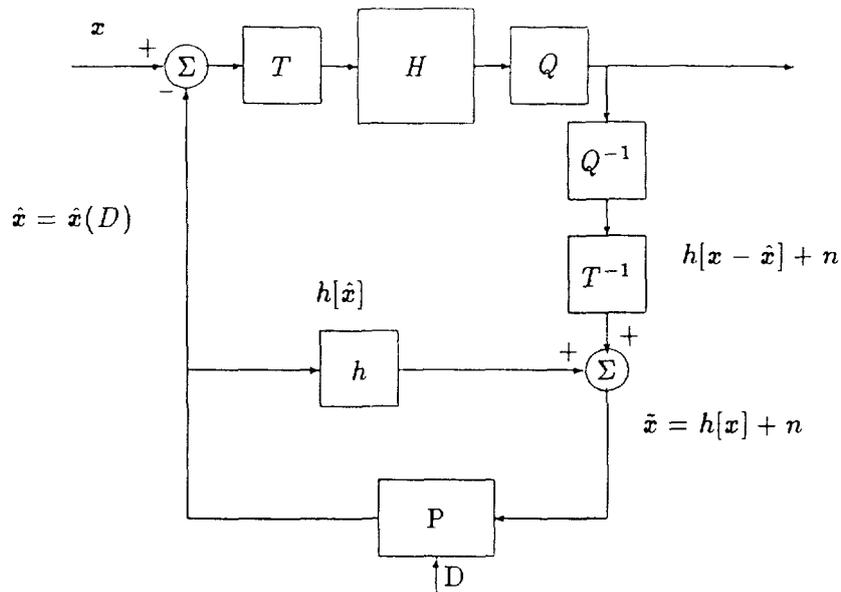
Figure 5: Filtering in reconstructed loop
