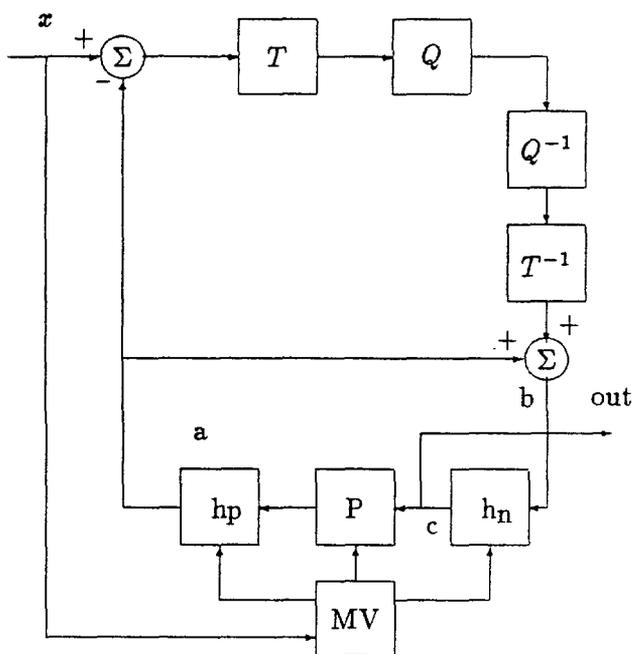
Figure 3: Structure of the source encoder
