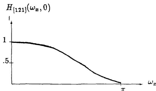
Figure 6: 1-D Transfer function of [1 2 1] filter
