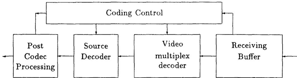
Figure 2: Structure of the receiver side
