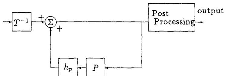
Figure 9: Position post codec processing in the decoder
