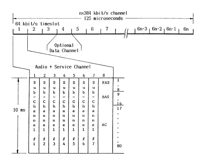
FAS: Frame Alignment Signal (note) BAS: Bitrate Allocation Signal
