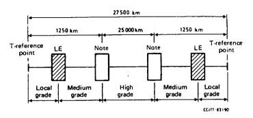
Note — It is not possible to provide a definition of the location of the boundary between the medium and high grade portions of the HRX. Note 4 to Table 2/G.821 provides further clarification of this point.
