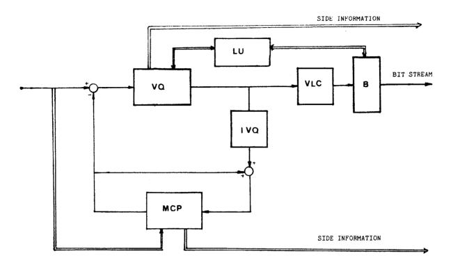
figure 1. VQ based hybrid codec
