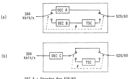
DEC A: Decoder for 525/60 DEC B: Decoder for 625/50
