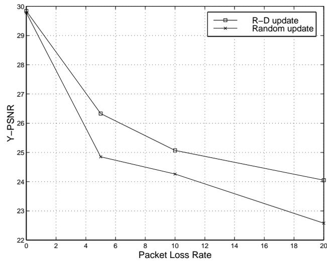
Figure 4: Performance of random vs RD optimized intra macroblock refresh with error concealment for the video sequence **COASTGUARD**.
