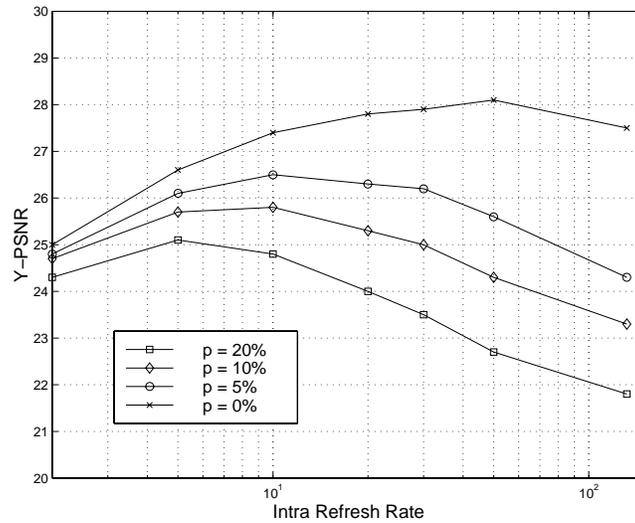
Figure 1: Performance of intra macroblock refresh with picture loss rate for **PARIS**.
