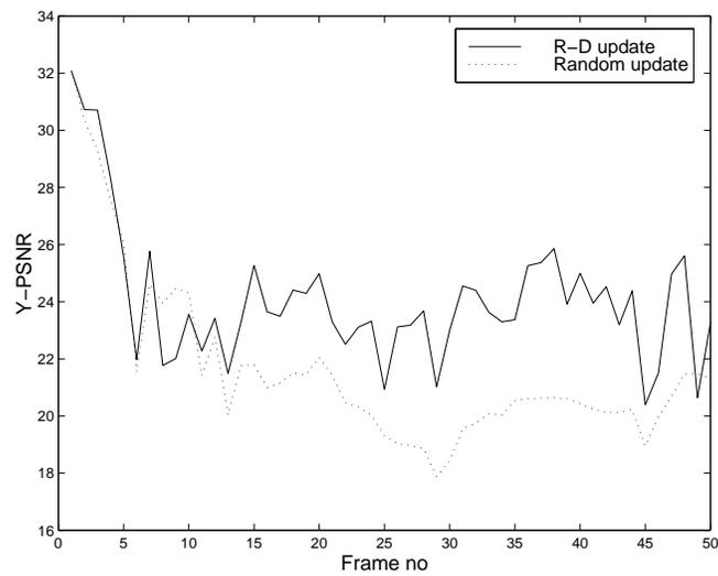
Figure 5: Performance of random vs RD optimized intra macroblock refresh with error concealment at a PLR of 20% for the first 50 frames of **FOREMAN**.
