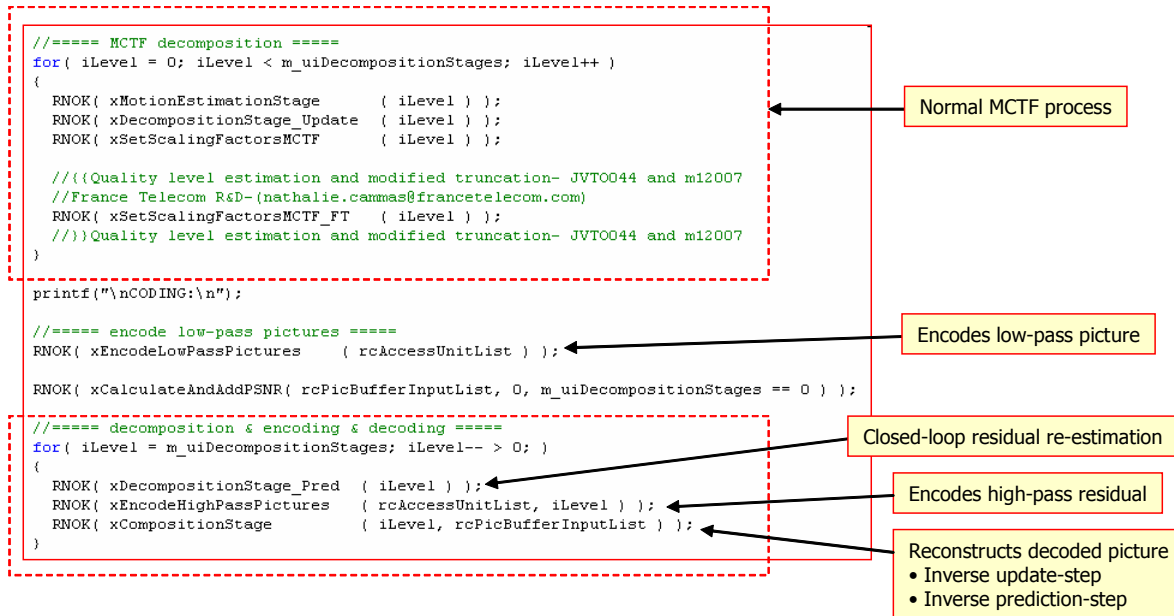
Figure 4 Closed-loop residual re-estimation in the context of MCTF process.
