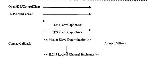
The Q.931 and H.245 protocol exchanges occur on two different reliable transport sockets. In each case, a WinSock modeled call sequence consists of the following steps.
