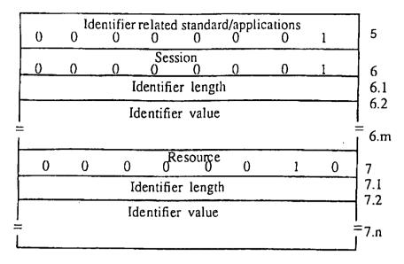
Figure - Coding of the Generic identifier transport IE for DSM-CC resourceId
