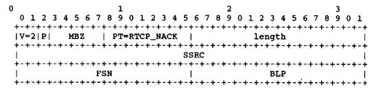
The various fields T, P, PT, length and SSRC are defined in the RTP specification [Annex A+]. The value of the packet type (PT) identifier is the constant RTCP\_NACK (193). SSRC is the synchronization source identifier for the sender of this packet.
