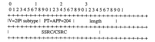
The APP packet is intended for experimental use as new applications and new features are developed, without requiring packet type value registration. APP packets with unrecognized names should be ignored. After testing and if wider use is justified, it is recommended that each APP packet be redefined without the subtype and name fields and registered with the Internet Assigned Numbers Authority using an RTCP packet type.
