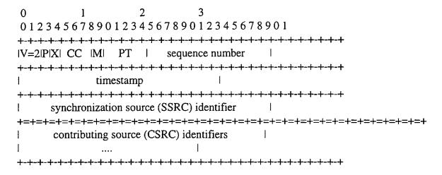
The first twelve octets are present in every RTP packet, while the list of CSRC identifiers is present only when inserted by a mixer.
