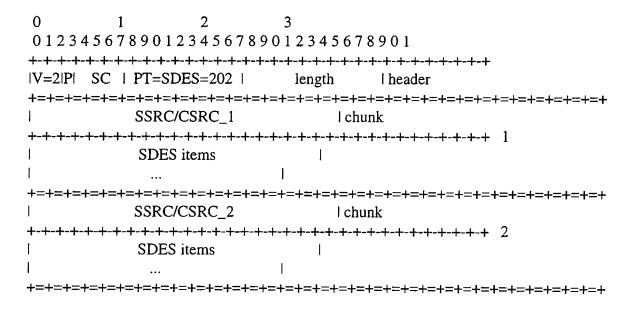
The SDES packet is a three-level structure composed of a header and zero or more chunks, each of which is composed of items describing the source identified in that chunk. The items are described individually in subsequent sections.
