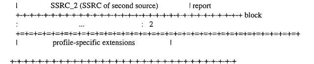
The format of the receiver report (RR) packet is the same as that of the SR packet except that the packet type field contains the constant 201 and the five words of sender information are omitted (these are the NTP and RTP timestamps and sender's packet and octet counts). The remaining fields have the same meaning as for the SR packet.
