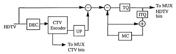
TQ: Transformation and Quantization ITQ: Inverse transformation and inverse quantization
