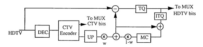
TQ: Transformation and Quantization ITQ: Inverse transformation and inverse quantization
