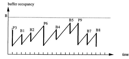
In this case, VBV removes the buffer contents for each irregular period. Therefore an encoder must control the coding operation carefully not to cause VBV violation.
