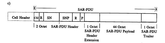
The SAR-PDU Trailer [in (a) and (c)] could incorporate protection for the SAR-PDU Payload by using FEC or a CRC. The Header Extension [in (b) and (c)] may be useful for signalling further information about the SAR-PDU Payload to the CS layer (e.g. Length Indication for partly filled cells).
