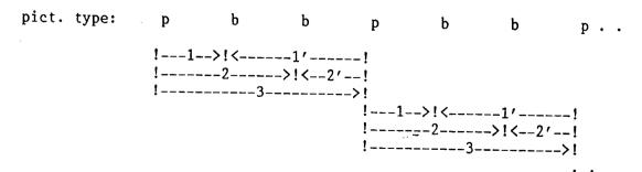
The prediction scheme for MPEG 1 in the proposed low delay I p'p'p'.. mode (interpolative prediction mode) looks like:
