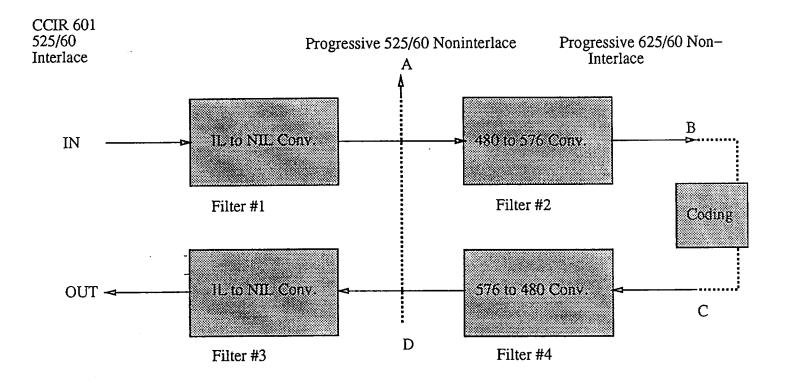
Figure 1a: Configuration of the Simulation System for SCIF 576 mode
