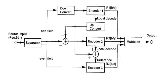
Fig.1: Encoder block diagram of HLPC
