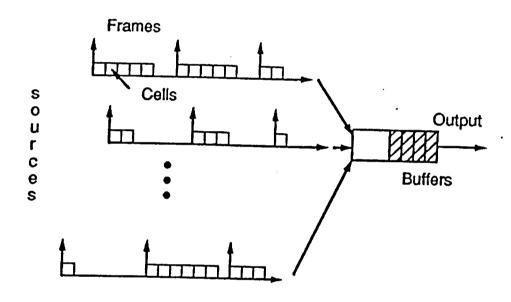
Figure 1. Single stage multiplexer
