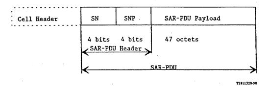
SN: Sequence Number (4 bits); to detect lost or misinserted cells.
