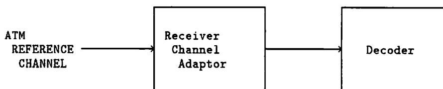
Figure 7.2: ATM Reference Decoder
