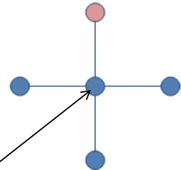
4-point connectivity used to determine edge pixel
