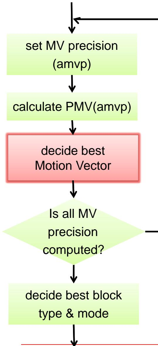
❖  $Mcost = Dist_{motion} + \lambda_{motion} \times (R_{amvp} + R_{mvd})$
