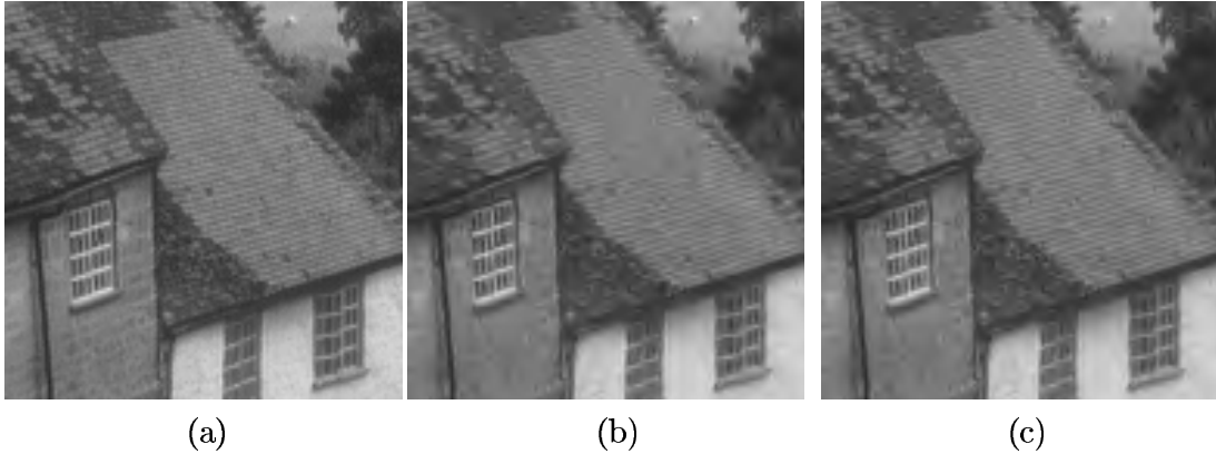
Fig. 5: Part of GOLDHILL: (a) Original (8 bpp), Reconstructions of (b) S&P-Coder[17] (33.13 dB PSNR) and (c) PACC-Coder (33.45 dB PSNR), both at 0.5 bpp.
