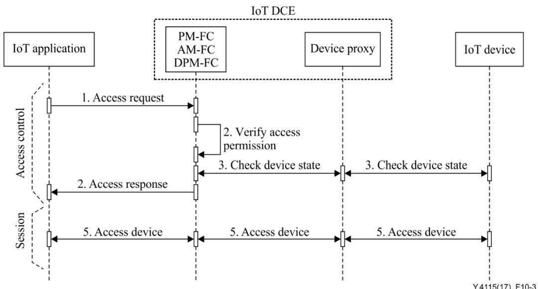
**Figure 10-3 – Flow for accessing to exposed IoT device capabilities**
