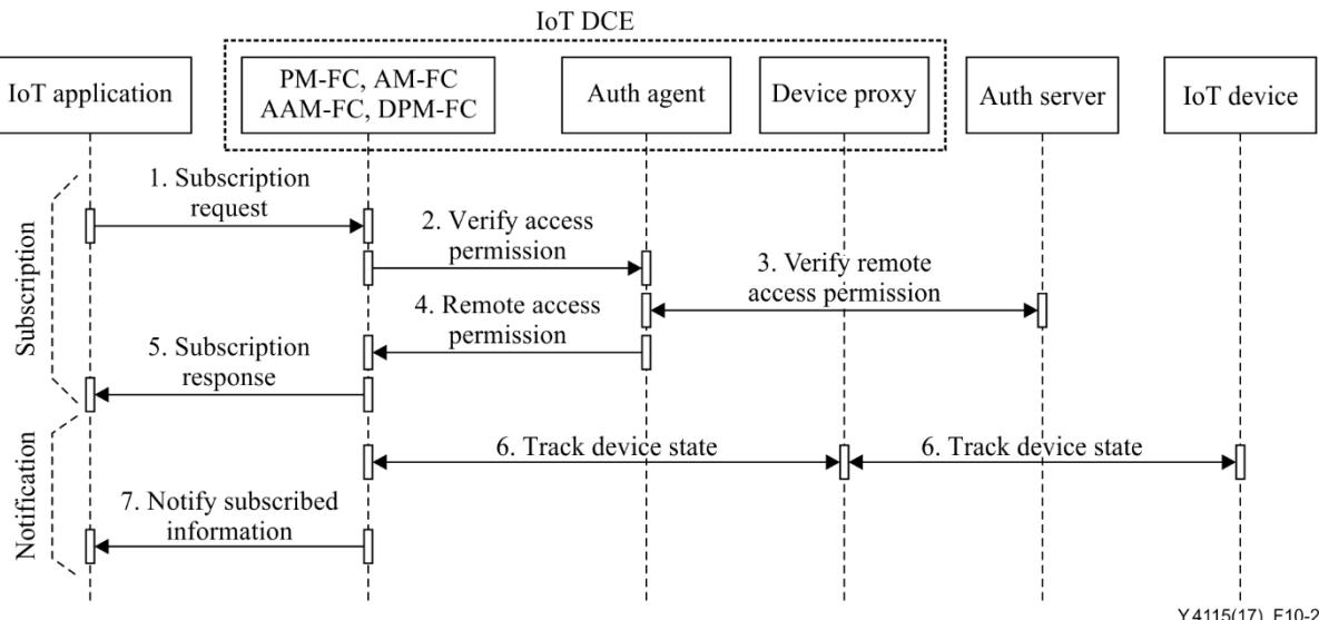
**Figure 10-2 – Flow for subscribing IoT device capabilities with remote access permissions**
