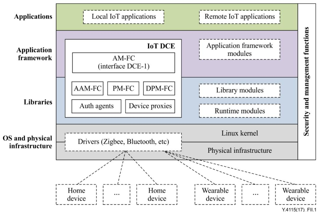
Figure II.1 – Implementation example of IoT DCE
