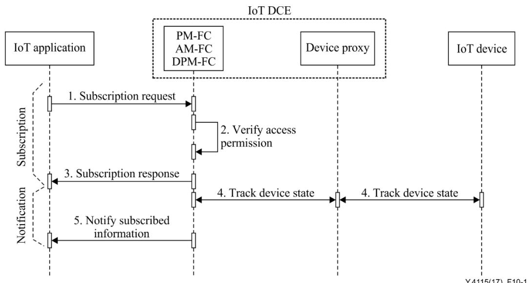
**Figure 10-1 – Flow for subscribing IoT device capabilities with local access permissions**
