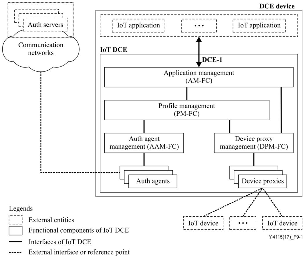
**Figure 9-1 – Reference architecture of IoT DCE**
