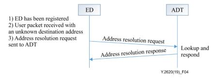
Figure 4 – Address resolution procedure
