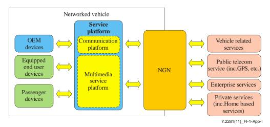
Figure I.1 – Service configuration model of a networked vehicle
