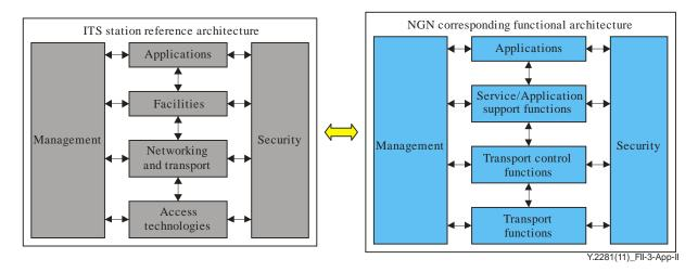
Figure II.3 – Correspondence between the ITS station reference architecture and the functions of NGN functional architecture
