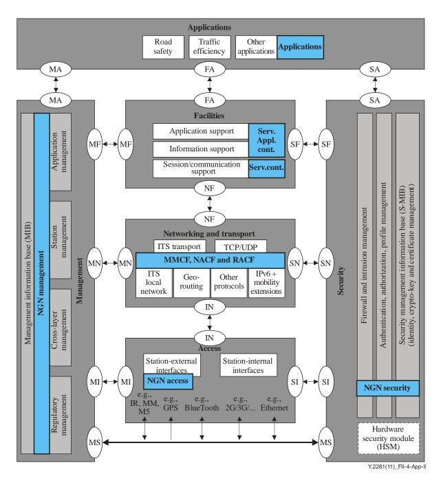
Figure II.4 – Arrangement of the relevant NGN functions into the ITS station reference architecture
