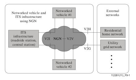
Figure 9-1 – Overall configuration model of networked vehicle and ITS infrastructure
