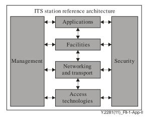
Figure II.1 – ITS station reference architecture
