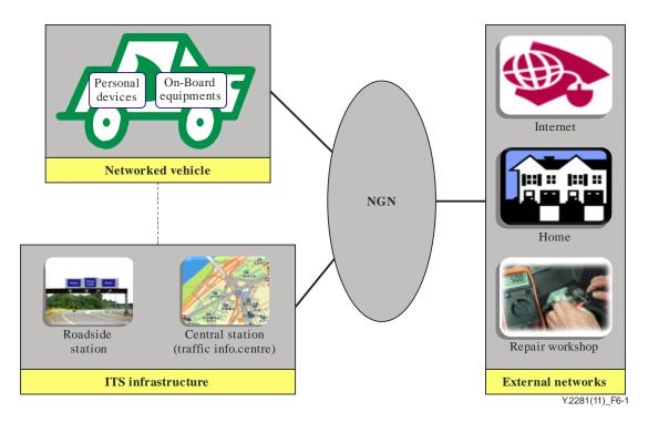
Figure 6-1 – High-level view of a networked vehicle using NGN capabilities
