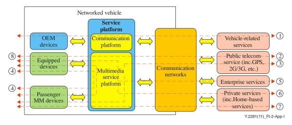
Figure I.2 – Classification of use cases for communication of a networked vehicle
