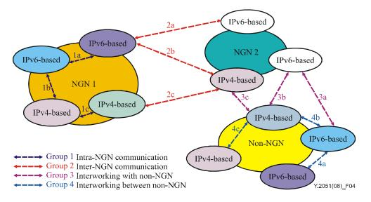
Figure 4 – Relationships of IPv6-based NGN with other IP-based networks
