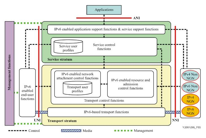
Figure 3 – Functional architecture of IPv6-based NGN
