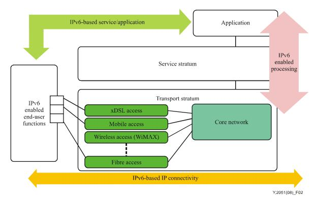
Figure 2 – Overview of IPv6-based NGN
