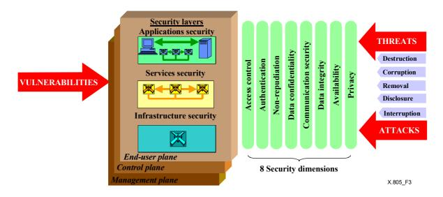
Figure 3/X.805 – Security architecture for end-to-end network security
