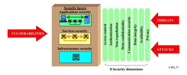
Figure 1/X.805 – Applying security dimensions to security layers
