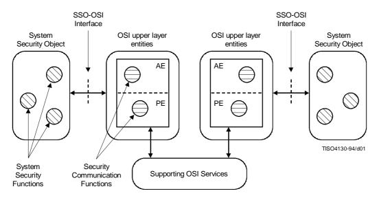
Figure 1 – Security functions associated with the OSI upper layers
