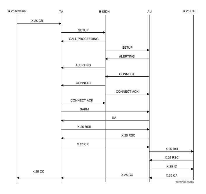
$FIGURE\ I.1/X.34$  Example message sequence for CALL SETUP
