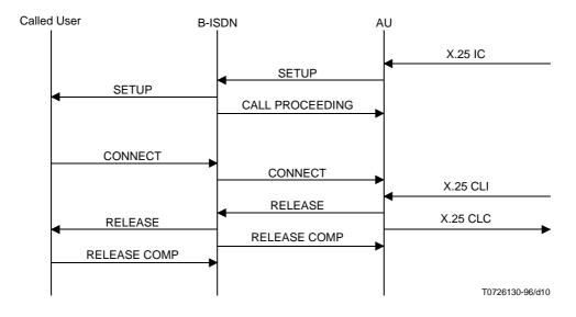
NOTE – After CONNECT message is received by the AU, there exists X.25 data link SETUP and restart procedures that are not shown in this diagram.
