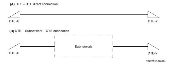
In case (B), there is no need, from the users' viewpoint, to consider the exact subnetwork configuration. The subnetwork may for example be: a single network, two interconnected networks (via an IWF or not), etc.
