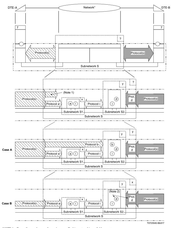
NOTE 1 – Depending on the use of case A or case B, this protocol is available or not. NOTE 2 – Not all elements of protocol "d" can be mapped to corresponding elements of protocol "a" used between DTE-A and subnetwork S1.
