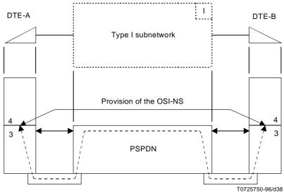
Example: PSPDN functionality for connection establishment, data transfer and connection release
