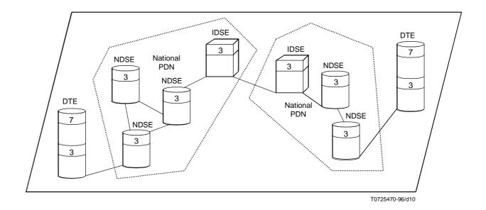
FIGURE 6-1/X.300 Example of an international PDN configuration with interworking
