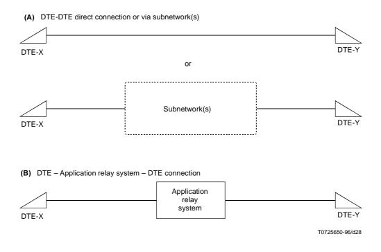
In case (B), there is no need, from the users' viewpoint, to consider the exact application relay system configuration. The application relay system may, for example, be: a single application IWF, two interconnected application IWFs, etc.
