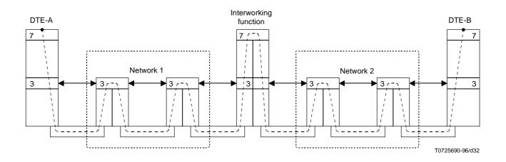
FIGURE 7-7/X.300 Interworking function at the application layer
