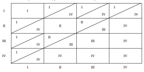
Different categories of interworking are defined in 6.2. Different types of subnetworks are identified in 6.3.1. Table 6-3b defines how the different categories are applied when interconnecting the identified subnetworks.
