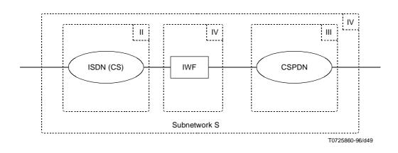
FIGURE B.9/X.300 Type IV subnetwork consisting of ISDN (CS) and CSPDN interconnected via an IWF
