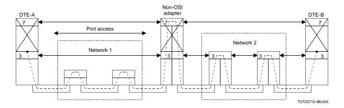
FIGURE 7-9/X.300 Interworking by port access via a non-OSI adapter
