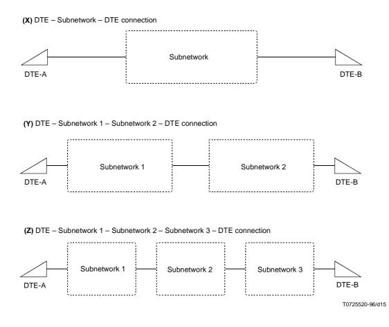
In cases (Y) and (Z), an IWF may be involved in any one of the subnetworks used. In case (Z), the intermediate subnetwork may consist of a single IWF.
