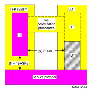
FIGURE 8/X.291 The RS test method
