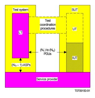
FIGURE 4/X.291 The remote test method
