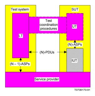
Note – The DS test method differs from the LS test method in that the upper interface of the (N)-entity under test is not a hardware interface.
