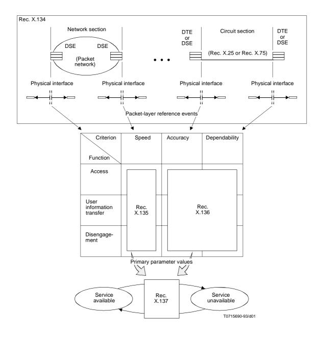
Figure 1/X.137 - Packet-switched service performance description framework
