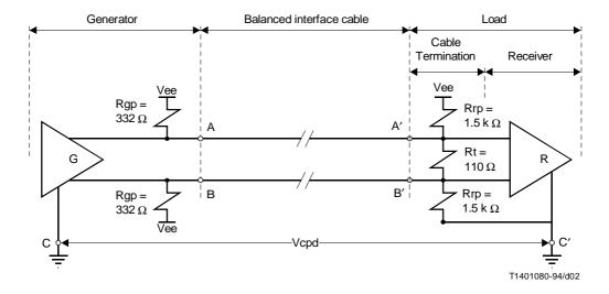
G Generator A, B Generator Interface Points Rgp Generator Pull Down Resistor A', B' Receiver Interface Points R Receiver С Generator Circuit Common Rt Termination Resistor C' Receiver Circuit Common Rrp Receiver Bias Resistor (Optional, Receiver Dependent)
