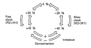
Note 1 – Phase measurements are given relative to R1 by the formula: Phase = phase(R2) – phase(R1). Note 2 – Receipt of a bit combination requiring an illegal move of more than one state will cause a legal move of one state in the appropriate direction.
