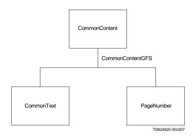
$\label{eq:FIGURE} FIGURE \ 7/T.502$  The common part of the generic logical structure
