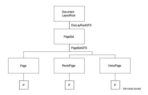
$\label{eq:FIGURE-8/T.502} FIGURE\ 8/T.502$  The layout structure – Document root and page sets
