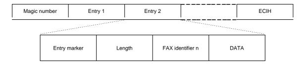
Figure 2/T.43 – Data structure of BCIH
