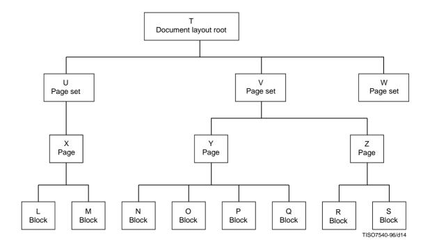
Figure D.9 – Layout structure of the document
