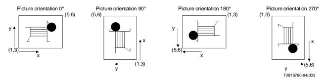
Figure 3 – Relationship of region of interest to the basic layout object (right handed axes)
