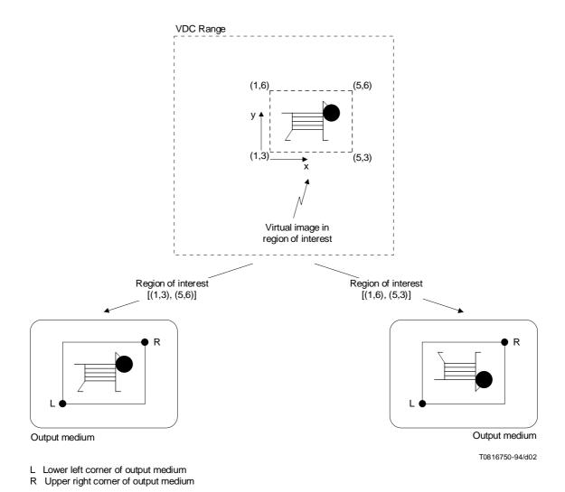
Figure 2 – Mapping of a virtual image defined in the VDC Space to an output medium (e.g. a softcopy device) using different region of interest specifications
