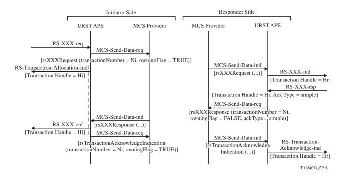
Figure 7-6 – Standardized acknowledged transactions sequence
