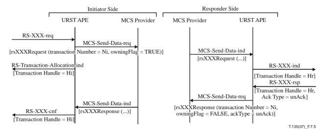
Figure 7-5 – Standardized unacknowledged transactions sequence
