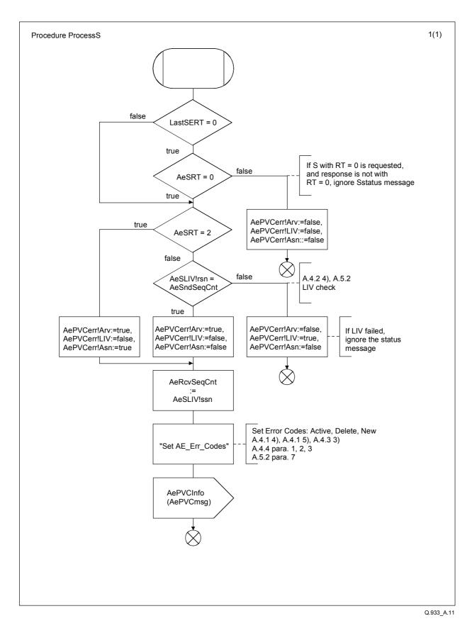
Figure A.11/Q.933 – Procedure ProcessS
