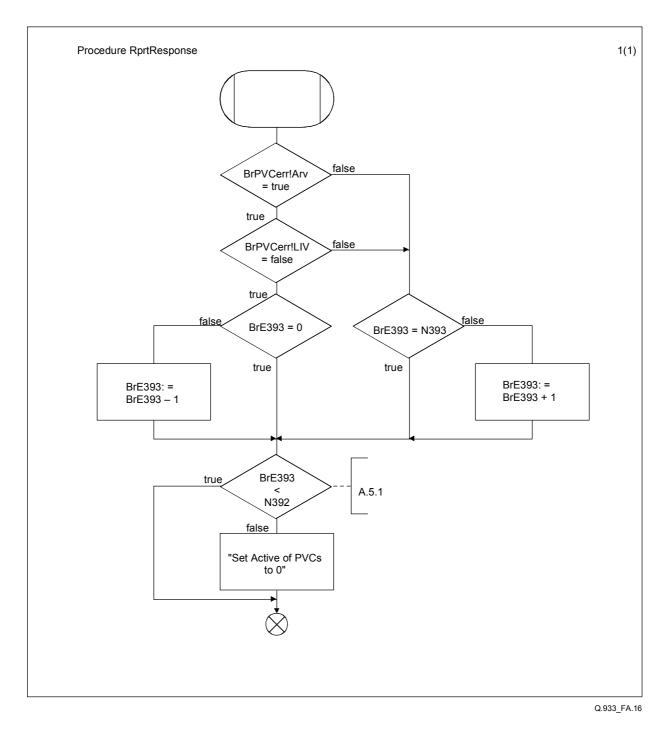
Figure A.16/Q.933 – Procedure RprtResponse
