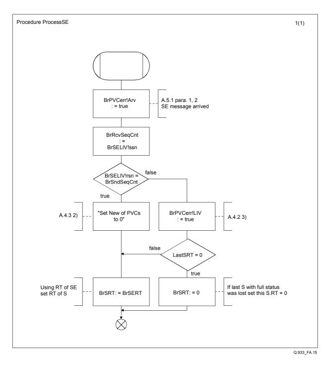
Figure A.15/Q.933 – Procedure ProcessSE
