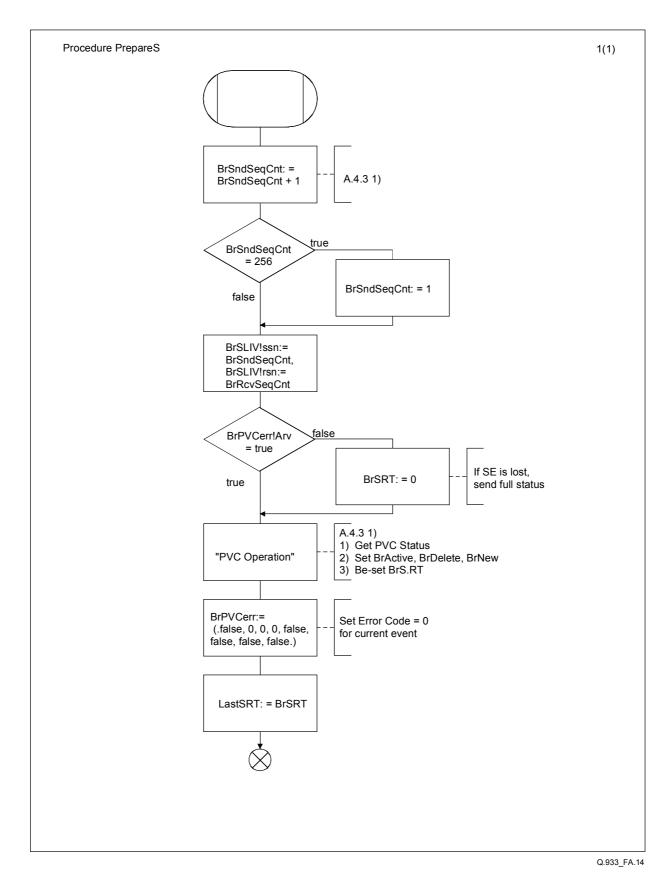
Figure A.14/Q.933 – Procedure PrepareS
